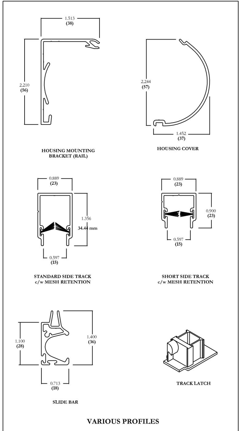
All Dimensions Are Shown In Inches and Millimeters In Brackets
